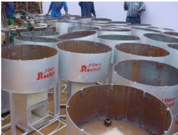
These stoves are lined with Dedza HTM-5 mortar. After three months of daily use, the High Temperature Mortar that lines the combustion chamber is still in tact.
