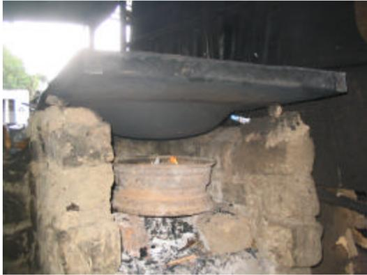
Due to the high cost of the chip frying pan (US\$15+) we decided to design a stove that could attach simply to the bottom of any frying pan. Andi Michel built a prototype but my understanding is that more work is needed on this design.
