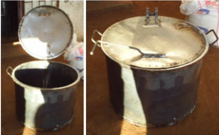
This is a pot made by Ken Steel Engineering. They feature a 3mm stainless steel bottom and 1.5 mm mild steel side and top. Although we would recommend using 1.5 mm and 3 mm stainless steel for all of the pot to ensure that it is durable, hygienic and long lasting (10 years+), this pot seems to fulfill the needs of schools and other
