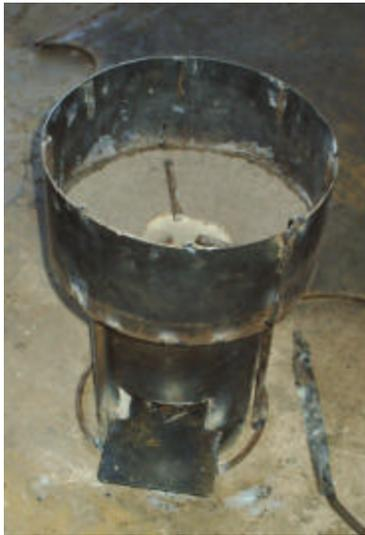
At least 6 Household Rocket Stoves were made in the spring of 2005. Three of these were made with Dedza bricks and the others were made with a mixture of fired and raw insulative bricks. For more info on these bricks please see Andi Michel's brief [report on homemade bricks](#).
