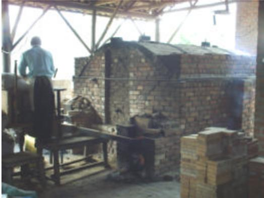
At present all of the insulative bricks that are used in institutional stoves in Malawi are made at Dedza Pottery. When transported with care and used correctly these sawdust/grog/clay bricks provide an excellent insulative refractory brick. Our goal is to build a combustion chamber for both the institutional and household stove that is light, refractory, insulative, and durable. Our focus for the household stove is **affordability** whereas our focus for the
