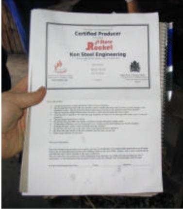
A comprehensive checklist (see [Quality control guide](#)) is used to ensure that each stove has been built to ProBEC's standards. Once this has been ascertained, the certificate is signed and dated and given to the purchaser. The producer's name and number are also printed on the certificate.
