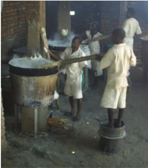
Since December 2004, five Metal Rocket Stoves have been in use (one retrofitted oil electric stove and four conical pot Rocket stoves) in the Maula prison kitchen. This has led to a greatly improved kitchen: no open fires, nearly smokeless cooking environment, and an incredible reduction in fuel consumption. **Maula prison has reduced its fuel consumption from 8 truckloads every two weeks to less than 1!** This also saves 900 Litres of diesel fuel each month.
