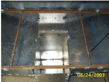
The baking compartment (2mm mild steel) is then inserted into the baking shell. Note the 2 cm gap on either side of the bread oven and the 4 cm gap on top of the bread oven.
