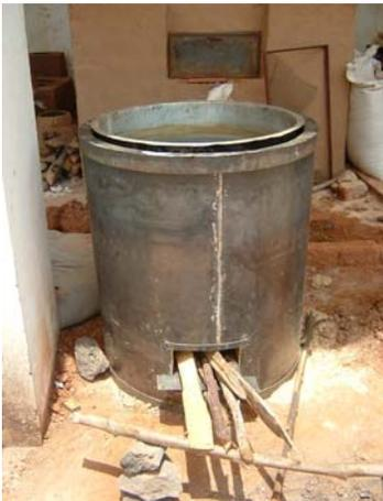
This stove is built around the same design as the fixed 100L version. The metal version, however offers an insulated double walled skirt so higher efficiencies would be expected
