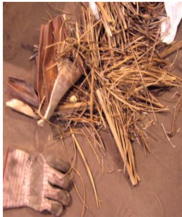
Pieces of coconut fronds (leaves) that can be combusted in a TLUD gasifier.
