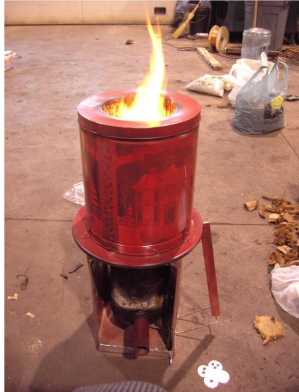
The disk in the bottom rises under the fuel canister, and is held in the raised position by the red stick on the outside. Note the metal controller of the primary flow.
