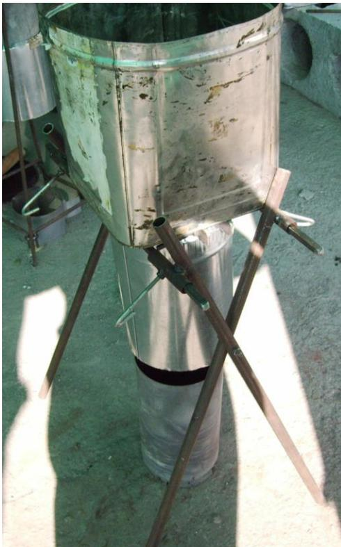
The “X” legs hold the horizontal bars that hold the stove’s upper body.
