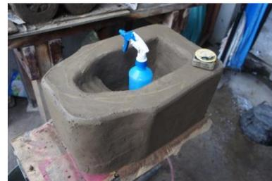
The Holey Rocket Stove with a char box as drawn and as built and now drying. Notice the pusher rod (center photo) and the char pocket (upper right photo) on which a can of sardines may fit at the cover and the char box (lower right). Another possible plug would be plaster of paris but should be built only after the stove was fired in the kiln to ensure a tight fit. .
